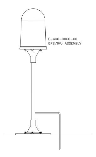
Figure 2–4. GPS/IMU Assembly
